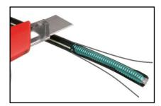
Remove 10 cm of the sheath to expose the cable body and ripcord. We recommend that you always use the ripcord to remove the sheath.
