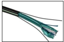
Make a small cut in the sheath with a wire cutter or sharp knife. Wrap the ripcord around the jaws on a plier.
