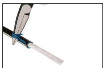
Remove the sheath and cut all the yarns and tapes lying around the fiber tube.
