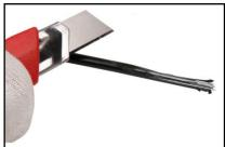
Remove 10 cm of the sheath to expose the cable body and ripcord. We recommend that you always use the ripcord to remove the sheath. Make a small cut in the sheath with a wire cutter or sharp knife. Wrap the ripcord around the jaws on a plier.
