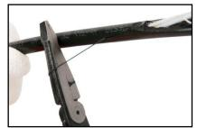
Remove the sheath and cut all the possible yarns and tapes lying around the fiber tube.
