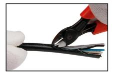
Put the ripcord in the small cut and pull it through the sheath. Keep the ripcord along the cable when opening the sheath.
