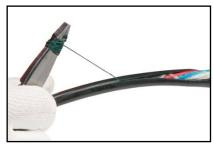
Remove the sheath and cut all the yarns and tapes lying around the fiber tubes. Unwrap the fiber tubes from the reinforcing member (FRP) and cut off the FRP in an appropriate length.
